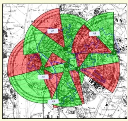
Decoupling by polarisation & frequency LOS nearly 100 % Reuse nearly 100 %
