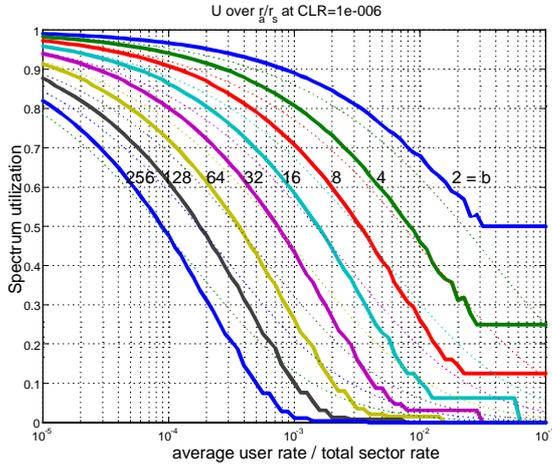
Figure 5: Spectrum utilization for a CLR of  $10^{-6}$
