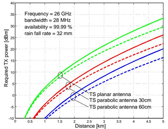
Figure 3: Required transmit power @ 26 GHz (depending on the terminal antenna type)
