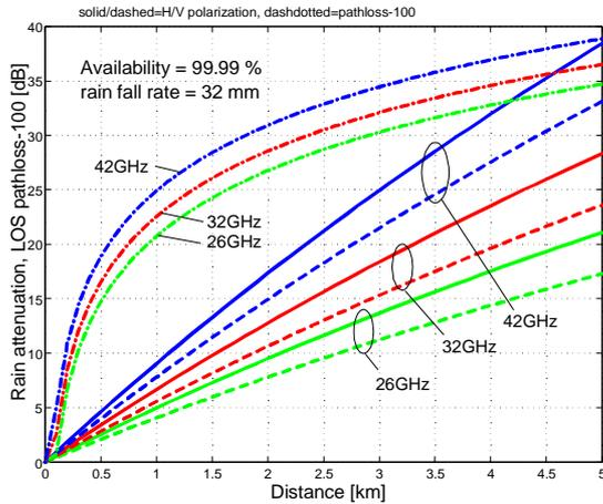
Figure 2: Rain fading @ availability=99.99% and free-space loss (depending on the frequency range)
