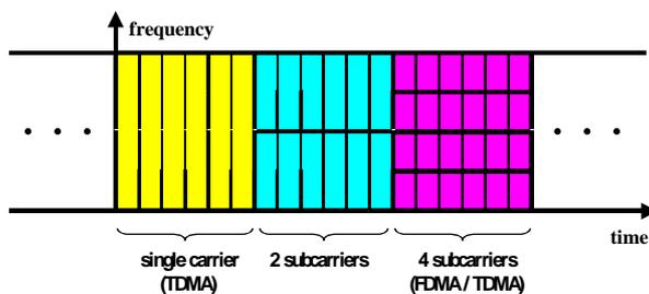
Figure 4: Hybrid TDMA/FDMA multiple access scheme for the uplink
