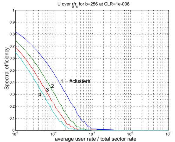
Figure 6: Spectral efficiency for  $b=8$  (top) and  $b=256$  (bottom) in case of user clustering
